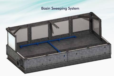
Thanks to our specially designed sweeping system installed in the tower basin, continuous water circulation is provided on the basin floor. In this way, the formation of sediment on the bottom of the tower basin is prevented, and the tower basin remains clean at all times. By preventing tower performance degradation, your tower will always remain clean.
